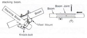
Fasten the wing nut firmly and screw in the knock-bolt until its tip screws in the boom.
